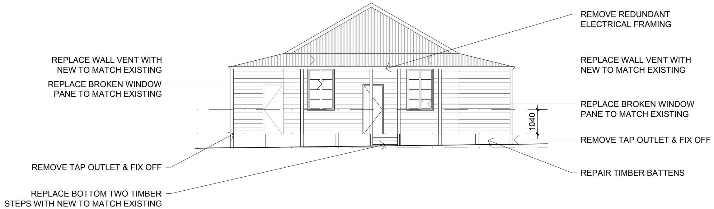
2 SOUTH EAST ELEVATION A24.20 B-24
