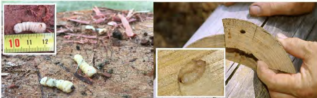
Left: Native longicorn beetle larvae, extracted from jarrah timber. Right: EHB larvae and a cross section of seasoned (dry) pine log showing larvae feeding tunnel.
